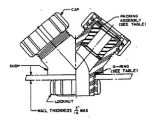
Each unit consists of body, caps, locknut and O-ring. Packing assemblies & neoprene plugs are available for all sizes.
